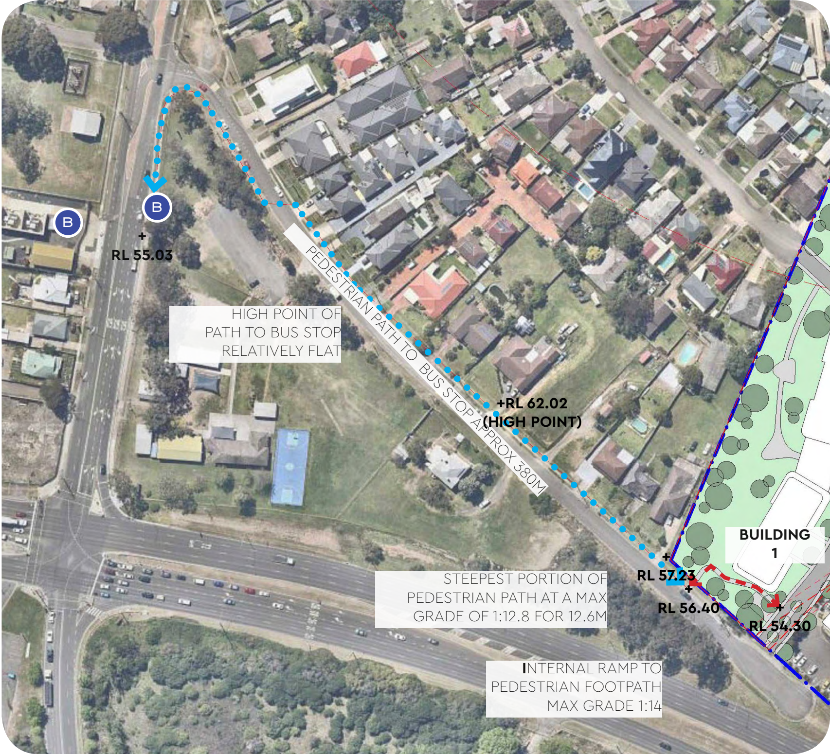
BUS ROUTE 2, GRADIENT FROM SITE BOUNDARY TO BUS STOP VARIES WITH STEEPEST GRADIENT OF 1:12.8 FOR 12.6M. FOR THE REMAINDER OF THE ROUTE, THE GRADIENT IS LESS THAN 1:14 WITH AN AVERAGE OF 1:20.5 FROM OUR PROPOSED ENTRY TO THE SITE TO THE HIGHEST POINT ON THE ROUTE AND AN AVERAGE GRADIENT OF 1:34 FROM THE HIGH POINT TO THE BUS STOP. THIS COMPLIES WITH SEPP WHICH ALLOWS AN AVERAGE OVERALL GRADIENT OF 1:14
